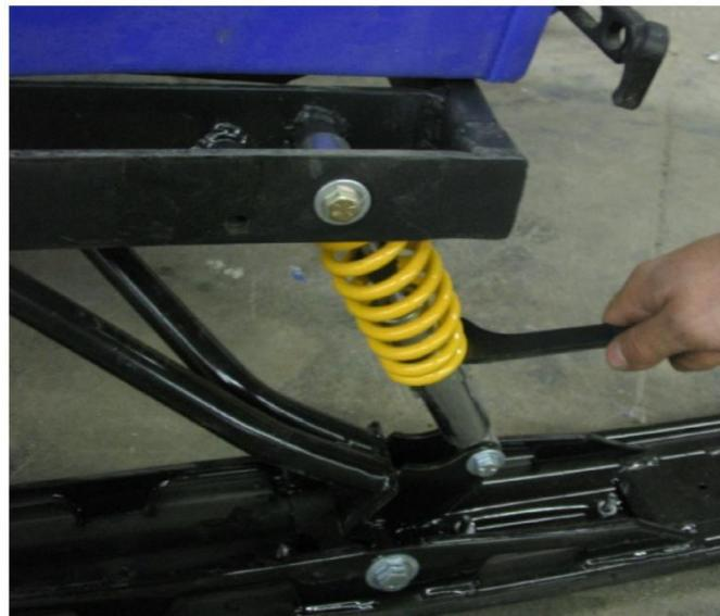
**Step 5:** Attach the hitch onto the Snowcoach frame with the four 3/8" x 1 1/4" fine thread bolts, eight 3/8" USS 17 Washers and four 3/8" fine thread nylon locknuts.
