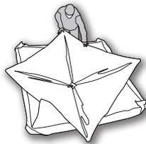
**Step 2:** Lay the ice shelter on the ground and check that there is no material twisted or overlapping the ends of any poles.
