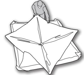
**Step 4:** Once the unit is lying flat, lift each of the corners together and stand the folded unit with all of the hubs facing down.
