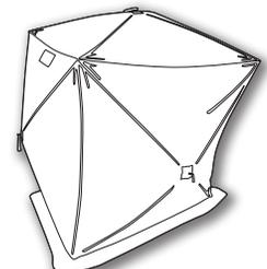
**Step 2:** Using your hand, push in centre hub on one outside wall until it collapses inward. Continue around the outside of shelter collapsing all remaining walls.
