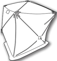
**Step 3A:** Pull outward on the loop on one of the walls. Continue around the entire shelter pulling each loop outwards on wall hub until all sides are popped out.
