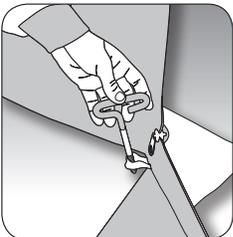
**Step 4A:** Position the shelter over fishing hole in ice and secure each loop on inside corners/walls of ice shelter to ice using the provided ice anchors.
