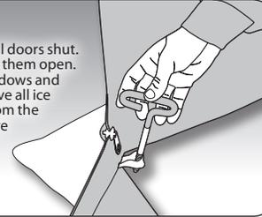
**Step 1:** Unscrew the ice anchors from the inside corners/walls and remove tie down(s) from the outside wall(s). Place all anchors and straps in the supplied pouch and store in the carrying bag.
